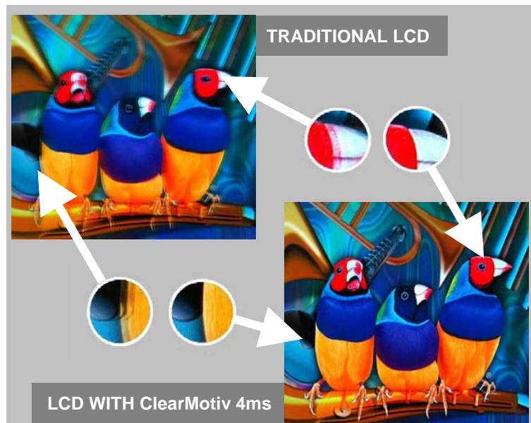
Figure 6: Traditional 8ms LCD vs ClearMotiv 4ms (10 pixels per frame)
